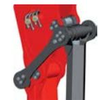
**LINKAGE SYSTEM** - Provides up to 60% more lifting power in the upper working area creating constant main boom speed and power throughout the lift.
