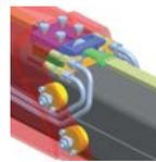
**EPSCOPE** - Extension components are located inside the boom for maximum protection. Service maintenance is facilitated by two protective covers that provide access to exchange hoses, pipes, and cylinder; no need to dismantle boom.
